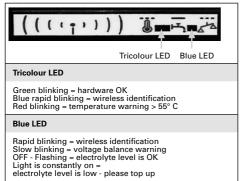
The Wi-iQ is the electronic device that communicates wirelessly to download the battery key information for better diagnostics & service. The device is fitted to a main DC cable on the battery to monitor and record data of current, voltage, temperature and electrolyte level (via optional external sensor). The LEDs on the Wi-iQ provide real time status of battery's condition.
