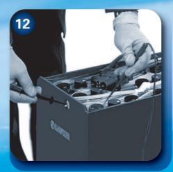
Measure insulation value Must be at least 50  $\Omega$  per V of nominal voltage.
