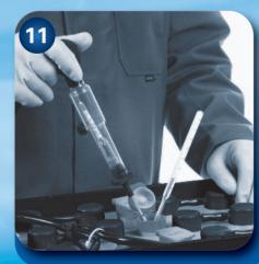
Measure electrolyte specific gravities and temperature If over 45°C, leave to cool down.
