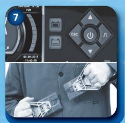
Switch off the charger Switch off the charger or check if the charger has been switched off. Disconnect the charger. Disconnect EC, if connected. Check final values if applicable.
