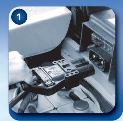
**Battery disconnect** Disconnect the electrical connection between the battery and the vehicle by separating the plugs.
