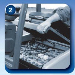
Remove the battery cover Leave vent plugs closed.
