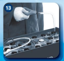
Clean the battery Clean the battery and extract liquid from inside the container!
