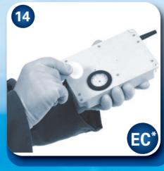
Exchange aeromatic filter Check air pump function.
