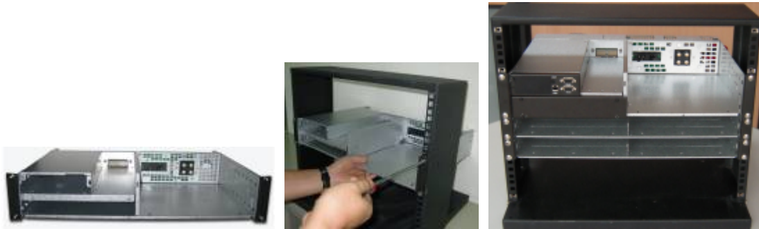
Figure 5—Mounting the STS chassis to the equipment rack
